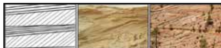
Figure 4. Cross bedding. Left: line diagram to illustrate simple cross bedding. Center: internal cross bedding of sand in a modern sand dune, which results from wind current deposition. Right: preserved cross bedding in sandstone of the Navajo Sandstone, which can be commonly found in Snow Canyon.
