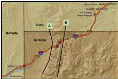
Figure 7. Representative faults. Fault "A" runs along the face of the mountains in Figure 3 at approximately mile marker 13. The desert floor to the west has been down dropped along this fault. Fault "B" crosses the interstate at approximately mile marker 18 and marks the boundary between the gray, tilted rocks and the brown and reddish flat-lying rocks.
